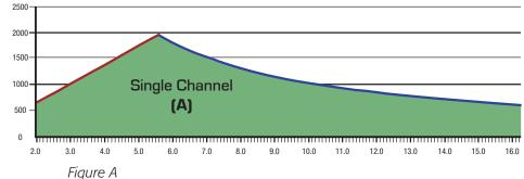
load. The graph (Figure A) demonstrates how a "normal" amplifier behaves. PLD and CXD amplifiers have the ability to deliver 100Vrms to the load, and can also deliver 17.7Arms to the load.
