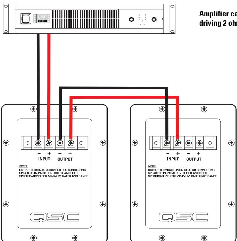
**Amplifier capable of driving 2 ohm loads**
