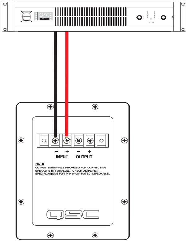
**Amplifier capable of driving 4 ohm loads**
