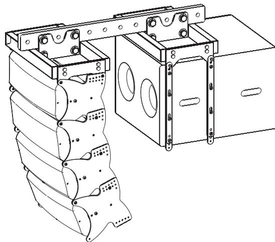
Figure 16: Using two PB2082-i Pull Back Bars for suspending a maximum of 4 WL2082-i loudspeakers.
