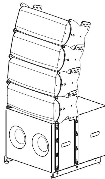
Figure 14: WL2082-i attached to WL115-sw and FB2082-i.
