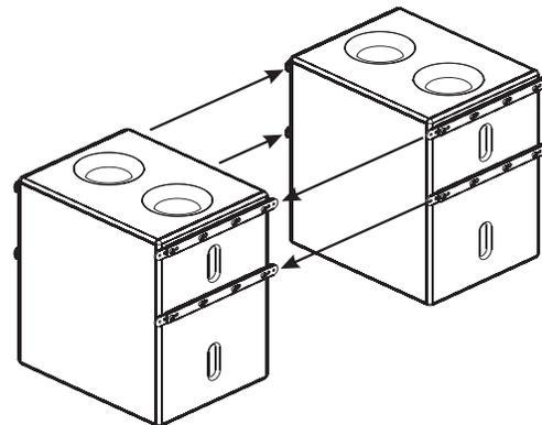
Figure 13: GS115-sw Ground Stack Rails attached to WL115-sw.
