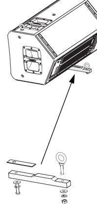
Pull-back bar assembly-Note location of offset cut-out on bar and orient to enclosure shape according to which side it is mounted on. Adhesive gasket is to be used between the bar and the enclosure. Ensure use of flat and lock washers in order shown. Tighten all hardware.
