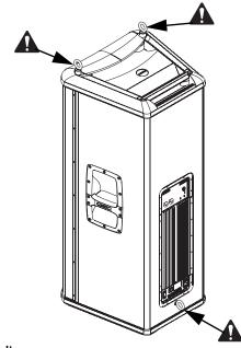
Before installing the eyebolts, remove the rubber inserts protecting the enclosure's threads (HPR152i and HPR153i only).
