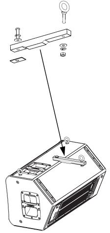
Installation of pull-back bar above the enclosure.
