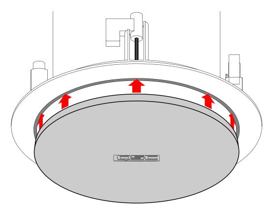
Then press the grille fully into the enclosure until it is fully seated. The grille is designed to compression-fit securely in place.
