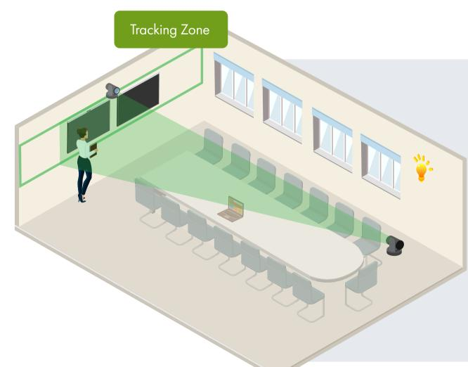
Al tracks 16-different points on the presenter's body, using data like height, clothing, and body movements.
