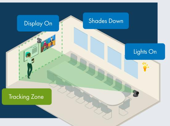
Creates a dynamic and responsive space tailored to the presenter's natural movement, with the Q-SYS Control engine allowing for an incredible range of movement-based automation.
