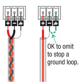
**Figure 1.** Left: Balanced connection; Right: Unbalanced with ground connection (most common type of unbalanced connection), or as "quasi-balanced" to avoid ground loops
