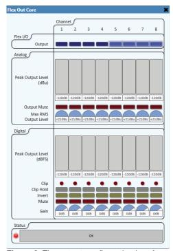
**Figure 3.** The output configuration box for the flex channels.
