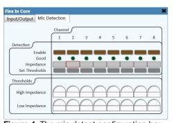
Figure 4. The mic detect configuration box.
