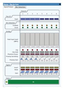
**Figure 2.** The input configuration box for the flex channels.
