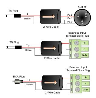
Figure 6 - Unbalanced Wiring Guide
