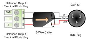
Figure 5 - Balanced Wiring Guide
