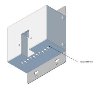
Access to the factory reset button is through a small circular hole on the underside of the unit, next to the ventilation cutouts.
