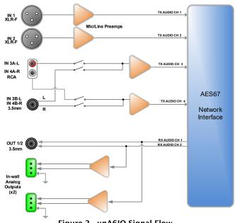
Figure 2 - unA6IO Signal Flow
