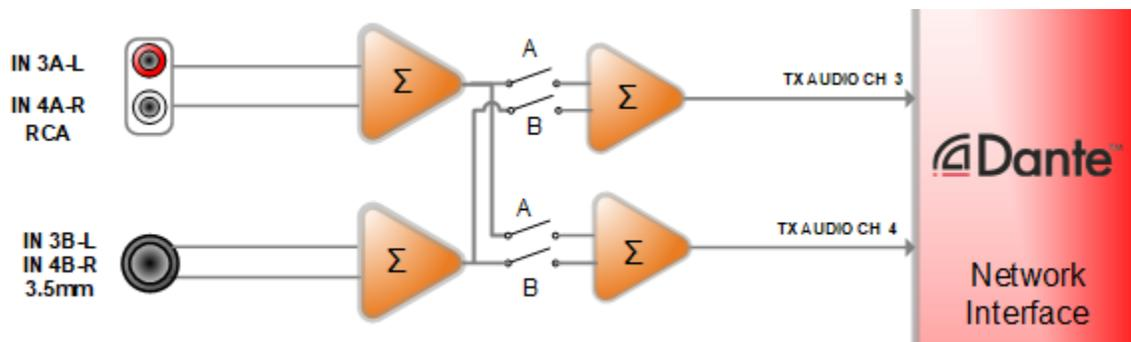
Older units prior to serial# 19070301-001 retain the stereo imagery so the input select for channel 3 selects which "Left" audio is selected for Dante channel 3 while input select for channel 4 selects which "Right" audio is selected Dante channel 4 (see below).
