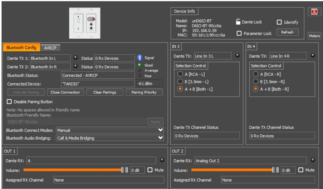
The configuration software for the unD6IO-BT is organized into the following key sections:
