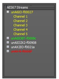
The AES67 stream list displays all AES67 streams that unIFY detects. It will includes streams from both Attero Tech devices and devices from other manufacturers. Each stream may be expanded to show the individual channels that stream contains.
