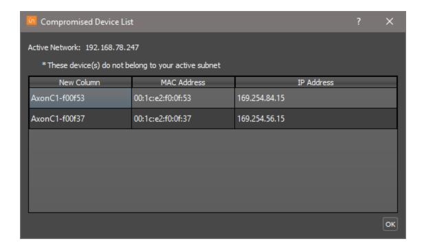
In order to communicate with these devices, change the IP address of the NIC that unIFY is using to communicate with the network to something that is in the same range of the device you want to communicate with.
