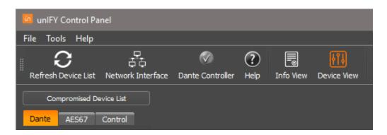
In order to communicate with devices over the network, the IP of the PC must be in the same range as the IP of the device. For AES67 and control devices, unIFY can detect if there is an IP address mismatch. When it does, unIFY will display, a "Compromised Device List" button.
