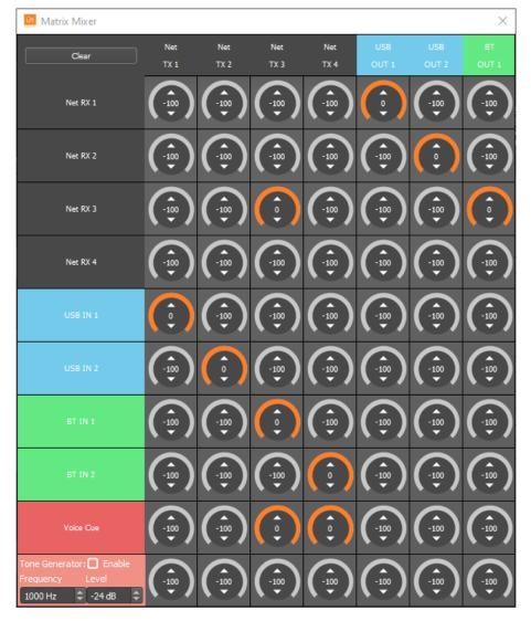
The mixer allows any input signal to be routed to any output signal with each cross point able to accept a value from -100dB to 0dB. Each cross point will show an orange level indication as the level is increased from -100.
