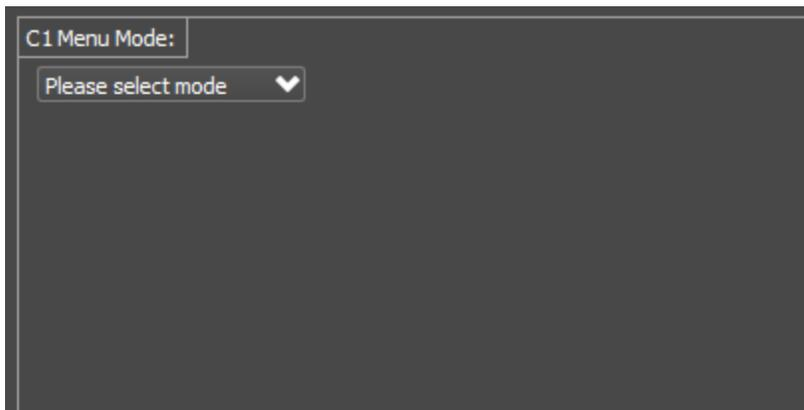
Before any configuration can be done, the C1 Menu Mode must be selected. The options are either "Q-SYS" mode or "3rd Party" mode. Use "Q-SYS" mode when the C1 is to be used with a Q-Sys Core DSP and will be married to a C1 plug-in using Q-Sys Designer. For everything else, select "3rd party".
