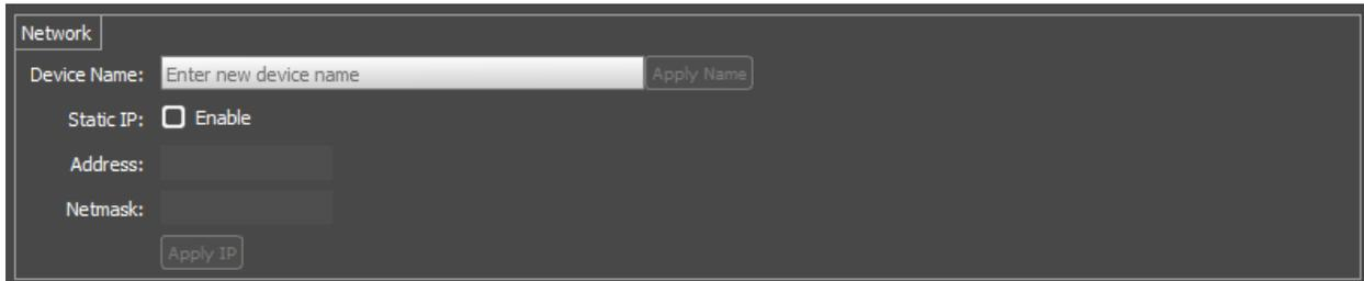
The network section allows customization of the devices name. By default this is AxonC1-xxxxxx where xxxxxx is the last 6 digits of the devices MAC address. The custom name can be a maximum of 16 characters long and must be unique among the C1's on a system.
