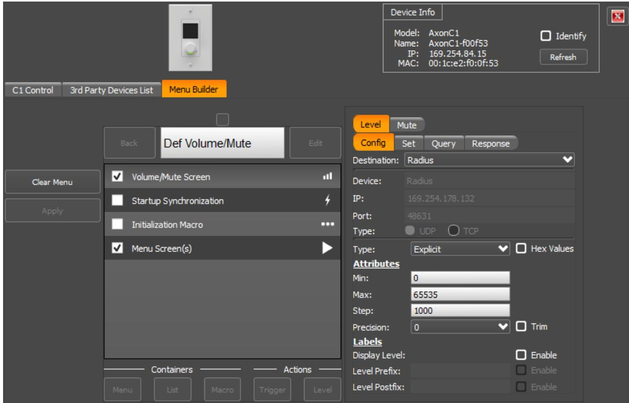
Each specific message the C1 sends is configured to be sent to a single specific destination. However the destination for different messages does not need to be the same. Essentially this allows the C1 to control different pieces of equipment if needed. The device list maintains a list of all the possible devices that a C1 needs to control. Each entry contains some basic information about how to communicate with that device.
