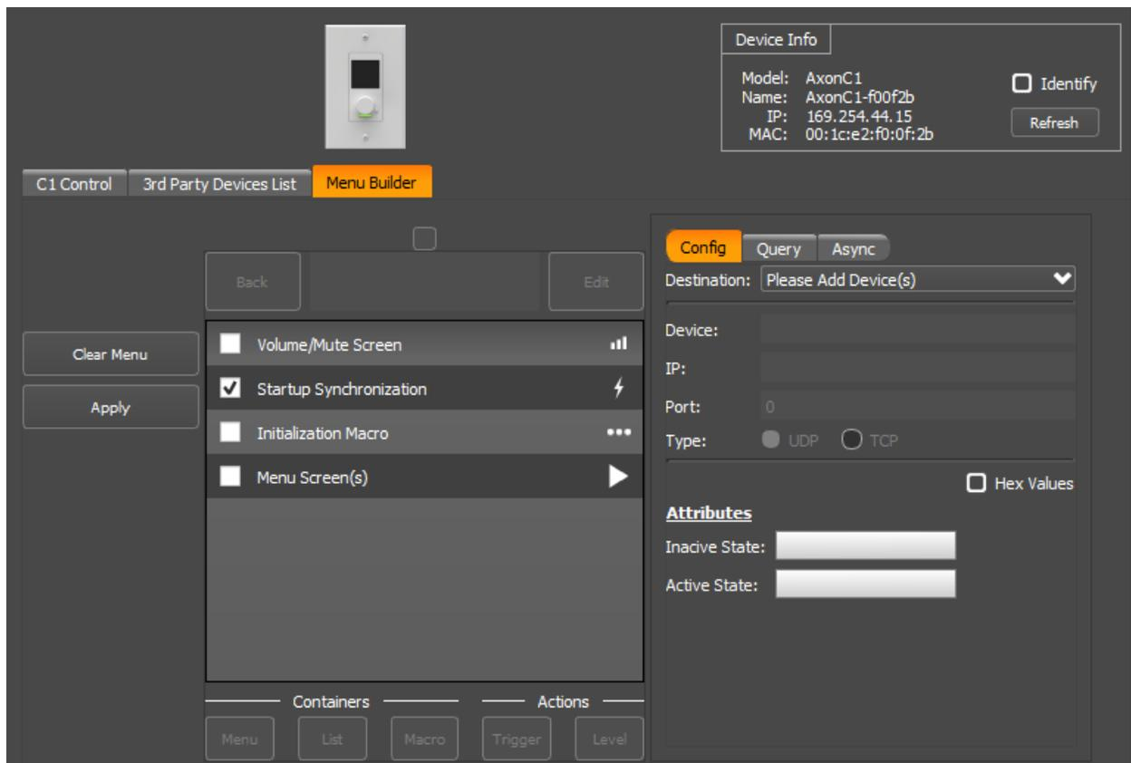
The "Async" tab configures how the C1 responds to asynchronous messages sent from the controlled device.
