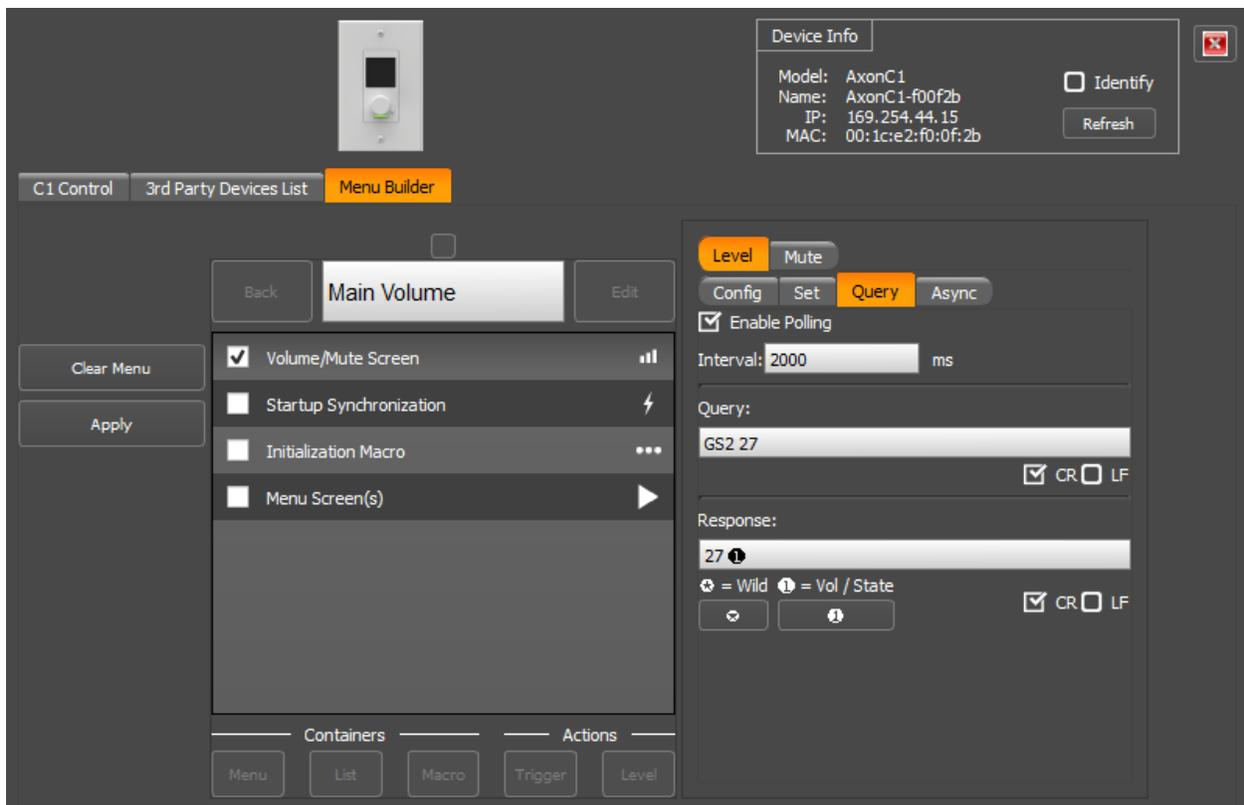
The screenshot displays the configuration interface for an Axon C1 device. At the top, there is a 'Device Info' section with the following details:
