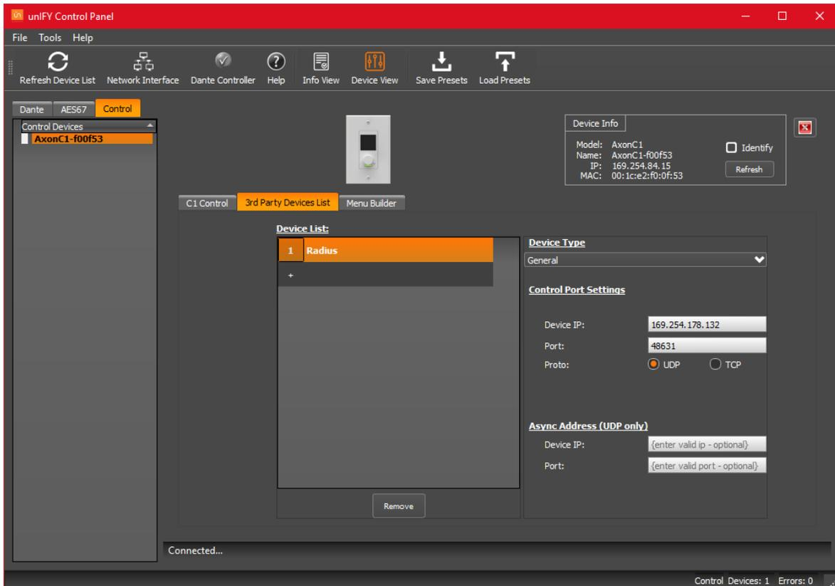
This allows a C1 to control a 3rd party device by sending UDP or TCP control messages to it. The exact makeup of those messages will be determined by the controlled device's API and the C1 will need to be programmed to send the correct command in the correct manner.
