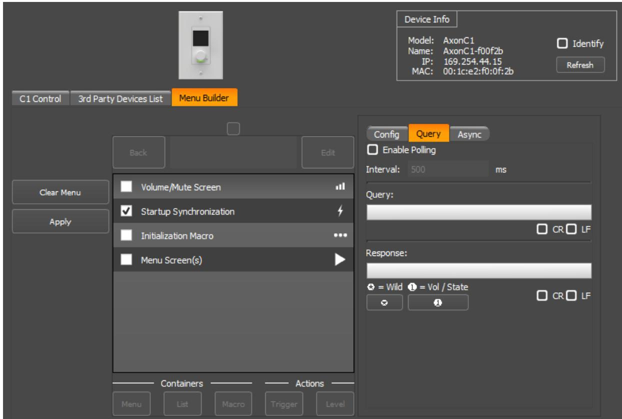
Startup synchronization options are used if, during C1 startup, the C1 needs to check if the device it is controlling is up and running before it starts any other communication. This can be done by polling it with a specific command at a pre-determined rate and/or waiting for the device to send a specific asynchronous message out.
