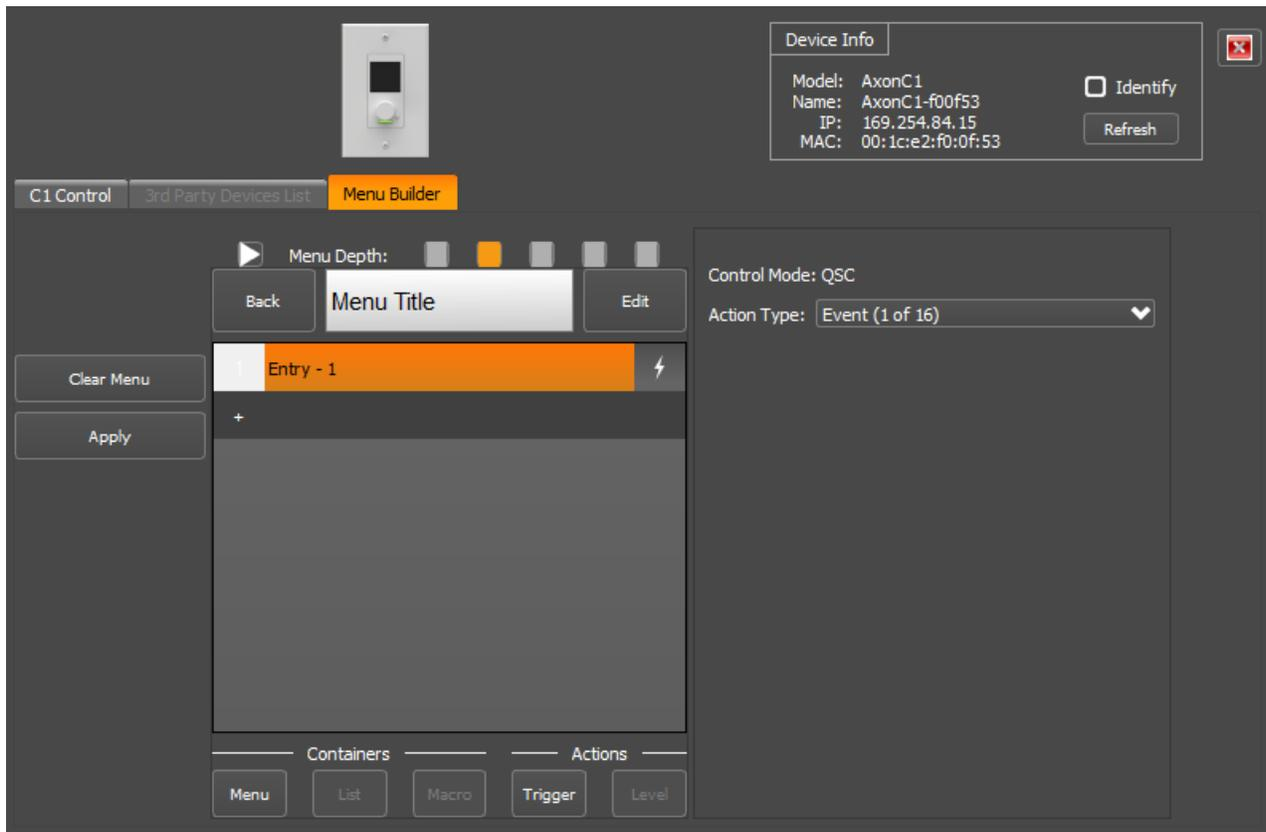
The menu builder allows the user to create a menu structure for events. The examples in this section refer to building a menu in Q-SYS mode.
