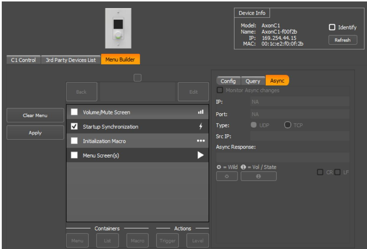
The "Async" tab configures the asynchronous messages the C1 is looking for to indicate the device is up and running correctly.
