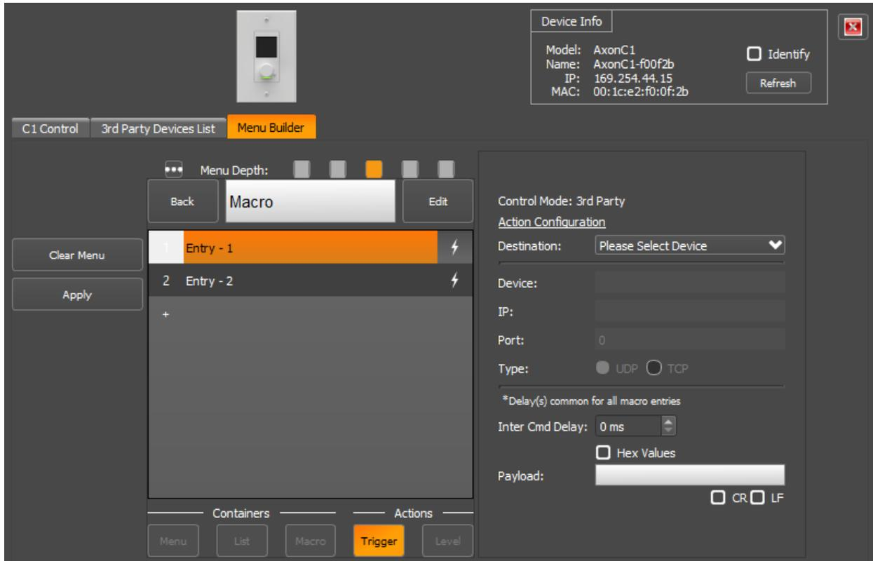
Triggers are used to send a single command to the specified target device to perform a desired action.
