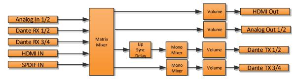
Figure 2 - Internal Audio Signal Flow
