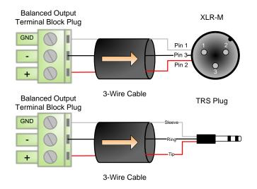
Figure 6 - Balanced Wiring Guide
