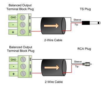
Figure 7 - Unbalanced Wiring Guide
