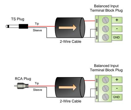
Figure 8 - Unbalanced Wiring Guide
