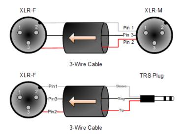
Figure 2 - Balanced Wiring Guide
