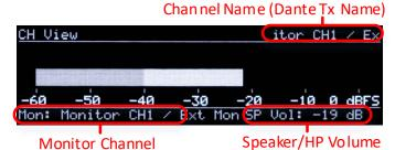
channels meter being shown is displayed in the upper left hand corner. The name in parenthesis that follows the name is the channel name that this channels is identified by on the Dante™ network. This view can also be used to select the monitor output if the front panel lock is not active. To do so, with the desired channel on view, click the "Monitor Select" button.
