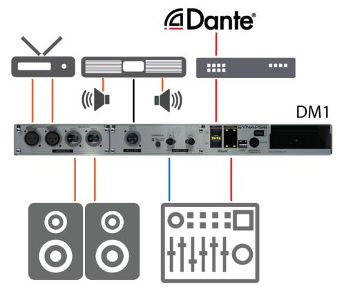
The Synapse DM1 is a rackmount networked audio monitor for confidence monitoring of networked audio and local sources via headphones or through the integrated speakers. The DM1 has 2 modes for network audio monitoring: *Standard and Extended*.
