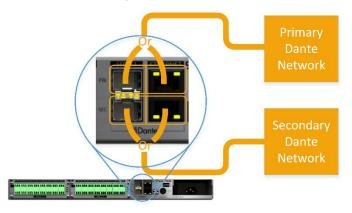
Figure 6 -"Redundant" mode, no daisy chain
