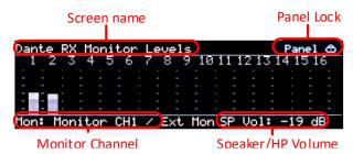
There are two views for bank metering. The main part of each bank view shows meters for each Dante™ input in that bank. This view can be used to select the monitor output if the panel lock is not active by pressing in the "Menu Nav" button. This activates a cursor that can be scrolled used the knob to select one of the visible channels. Once the desired channel is selected, press the separate "Monitor Select" button and that channel will when be routed to the speakers/headphone outputs.
