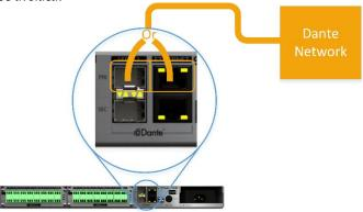
Figure 8 - "Standalone" connection in "Redundant" mode
