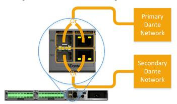
Figure 4 -"Redundant" mode, no daisy chain
