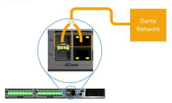
Figure 6 - "Standalone" connection in "Redundant" mode
