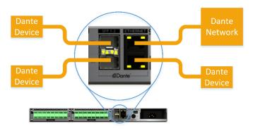
Figure 7 - "Standalone" connection in "Switched" mode
