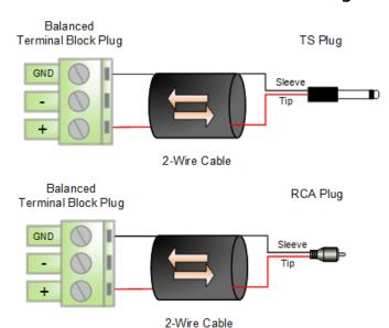
Figure 3 - Unbalanced Wiring Guide
