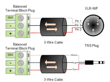
Figure 2 - Balanced Wiring Guide
