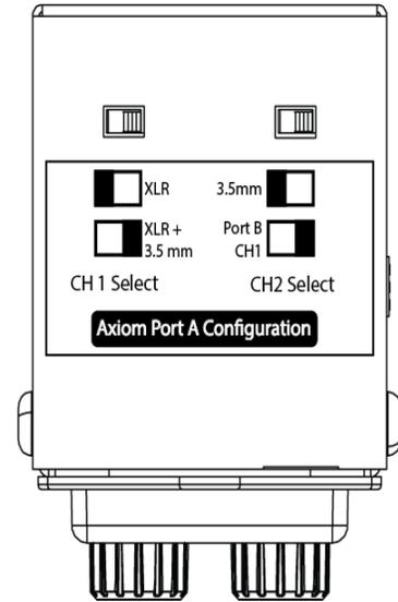
**CH 1 Select:** route either the XLR or a sum of the XLR and 3.5 mm inputs to the CH 1 output of Axiom Port A (on the AXP20).
