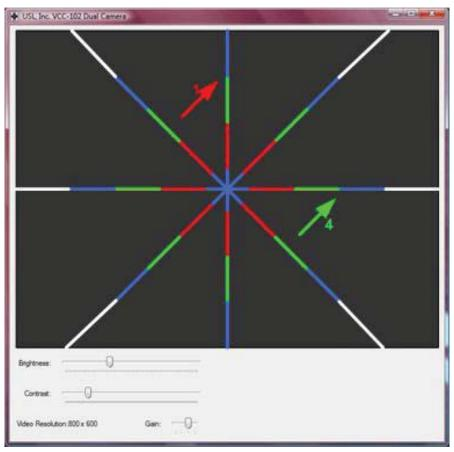
Video image focus is controlled by turning the threaded front adjustment ring to bring convergence pattern images into focus between the ranges of 20 feet to 150 feet. A top mounted red laser enables the technician to quickly locate the pattern on the movie screen.
