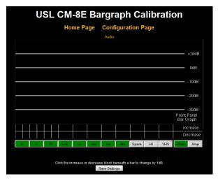
Play pink noise on a channel at reference level. Select only that channel using the front panel or web buttons. A bar (or two for biamp) should appear above the button corresponding to that channel. Click the mouse in the top box above the button to increase the height of the bar and the bottom box to decrease the height of the bar. As shown in the image above, when a
