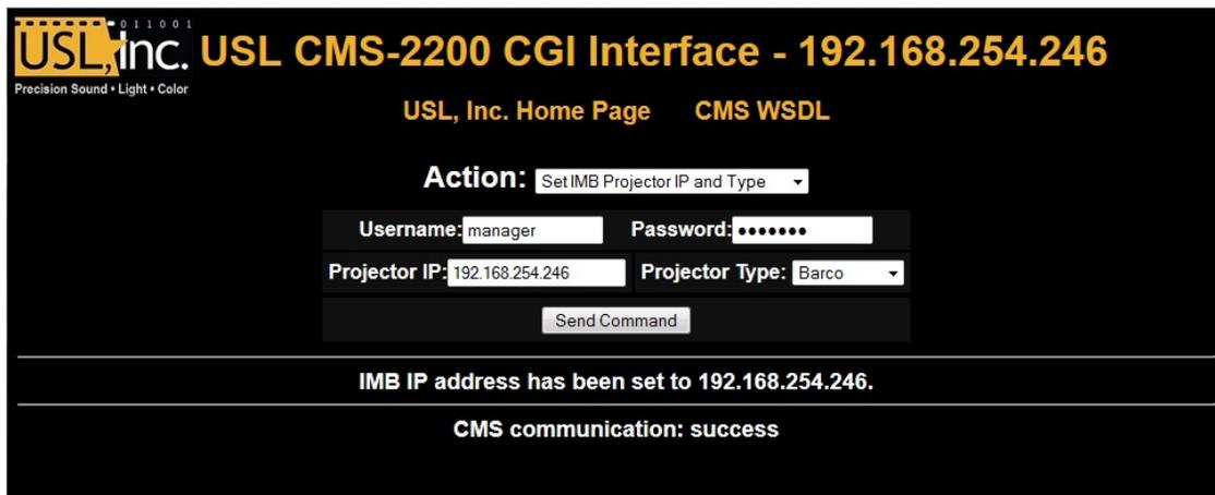
Figure 12-4. Set Projector IP Address and Type
