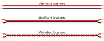
Figure 1. Reduce the loop area of loudspeaker cabling by using twisted pair wire.
