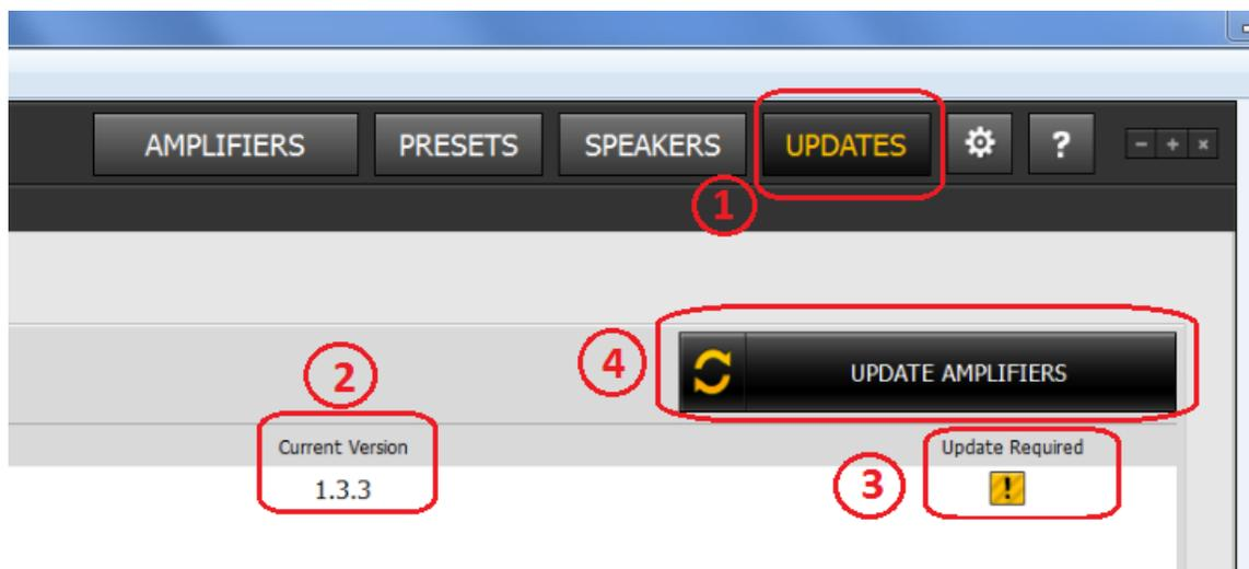
**Figure-1: Checking "Current Firmware Version" and "Update Required" status**
