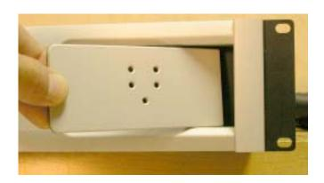
**2-** While lightly pressing the right side of the cover against the chassis, use the hex key tool (inserted into the plate's screw hole) to slide the cover to the left until the LEDs line up with the cover's holes. Continue to lightly press the cover against the chassis while you insert the cover's retaining screw and secure the screw. Fully tighten the retaining screw.
